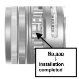
It is necessary to fill the space between UCL-90 LD and housing port with water, so <u>attach UCL-90 LD underwater</u> or <u>partially unscrew the lens allowing inside air to escape then retighten</u>.
